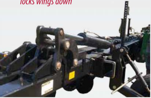
Pin-free, over-the-center design locks wings down
